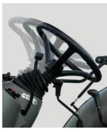
The adjustable steering wheel allows easy access and exit from the cab.
