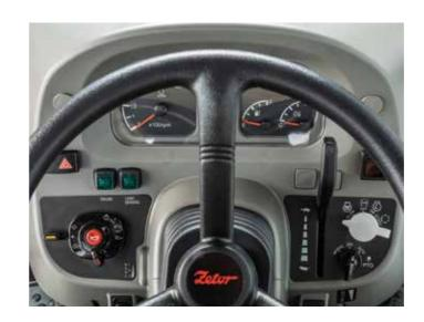
The easy-to-read LED dashboard displays basic operating data, such as engine speed, temperature, fuel level, time, PTO, etc.
