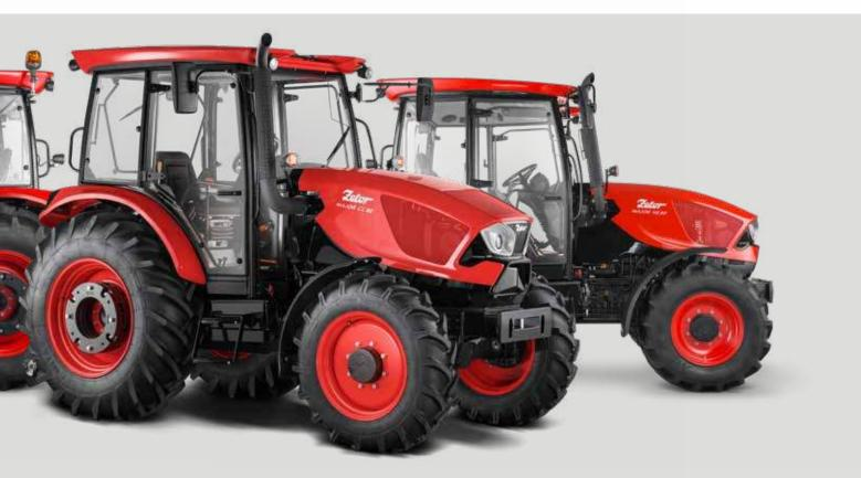
ments of more demanding customers. The cab is equipped with a more comfortable seat, passenger seat and storage compartments. The higher lifting force makes it possible to aggregate the tractor with more implements. The MAJOR HS's capabilities are best appreciated when working with the front loader.
