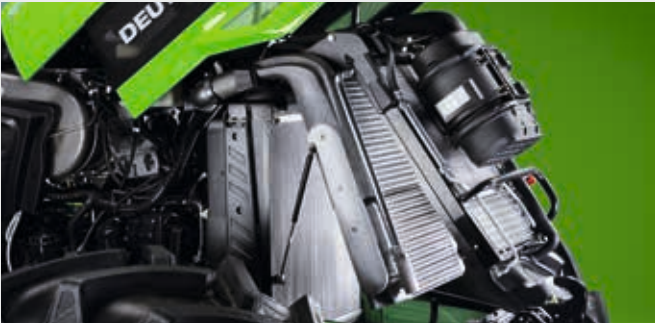
Long service life: redesigned radiator unit made from aluminium, opens fully for easy maintenance.
