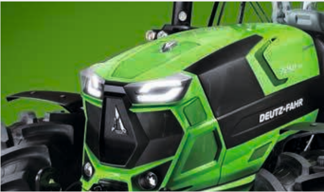
LED package with up to 40,000 lm.
