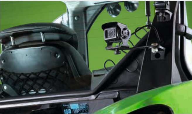
Integrated camera with automatic full screen mode (e.g. reversing) for overview and safety.
