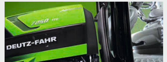
📌 Cab and bonnet are separated to reduce noise and vibration and increase comfort.
