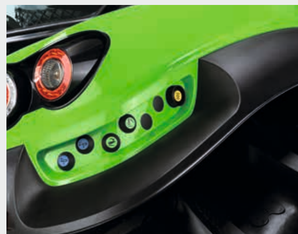
External operation for hydraulics, rear linkage and PTO.
