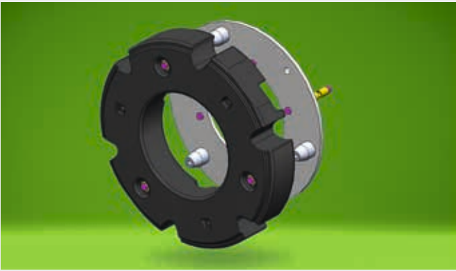
Rim ballast with up to 1,840 kg ballast weight.
