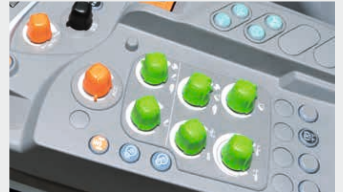
↑ ... as well as the controls for the front and rear linkage.
