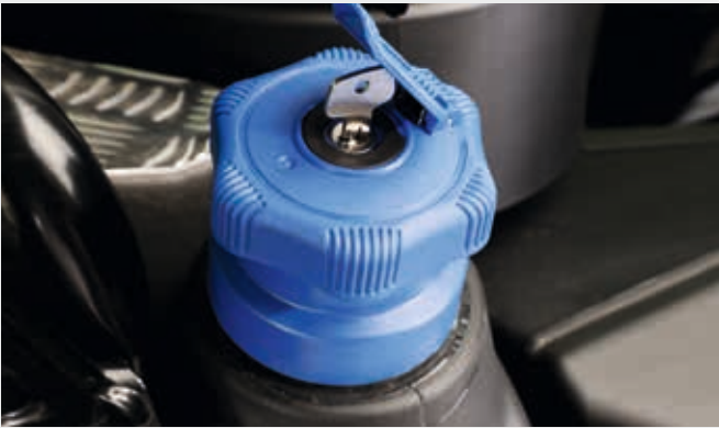
Lockable tank covers for fuel and AdBlue tanks.
