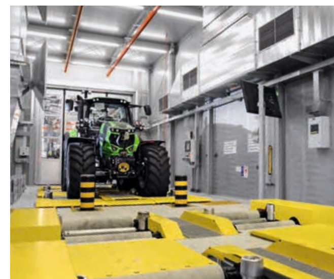
📈 Unique in tractor manufacturing: chassis dynamometer and axle suspension test bed.
