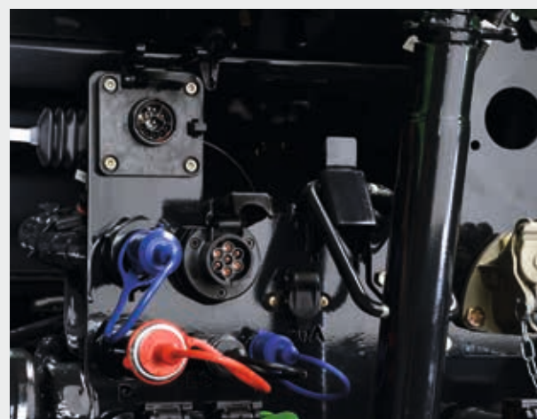
Convenient: ISOBUS interfaces at front and rear.
