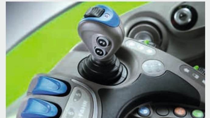
↑ The hydraulic valves are actuated with a joystick with an integrated thumbwheel.
