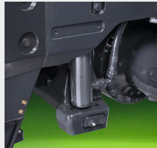
Unique new suspension concept for the front axle.
