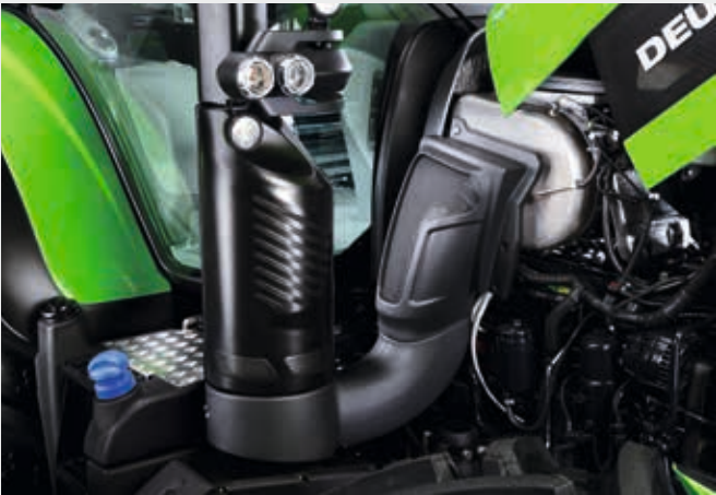
SCR exhaust gas treatment and passive DPF save fuel and operating costs.
