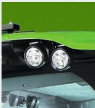
↑ Up to 16 LED work lights (generation IV, 2,500 lm per light).
