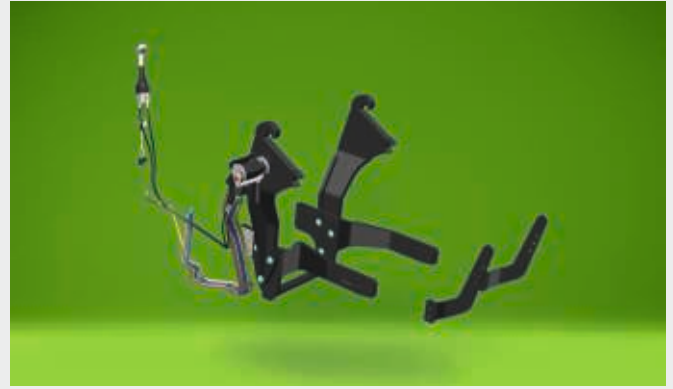
↑ With the Light Kit or Ready Kit, the interfaces for the front loader are already fitted on the tractor.
