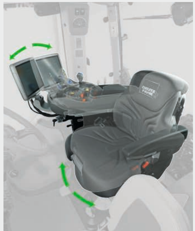
↑ Now available for all TTV models: Seat with up to 20° rotation for added comfort and ease of operation.
