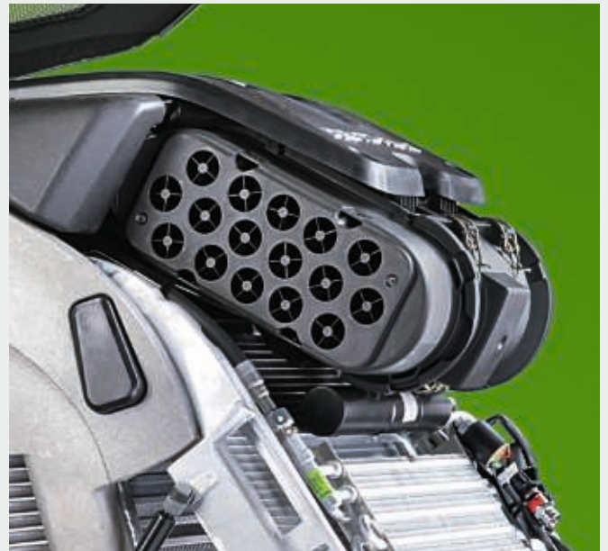
↑ Pre-cleaning system in the engine air filter: Spiral cyclone tubes and an aspirator hoses removes 95 % of the dust before these can enter the primary filter.
