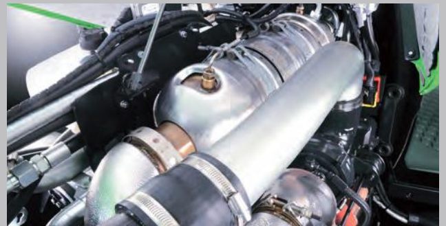
... and a diesel oxidation catalyst (DOC) catalytic converter guarantee minimum emissions.
