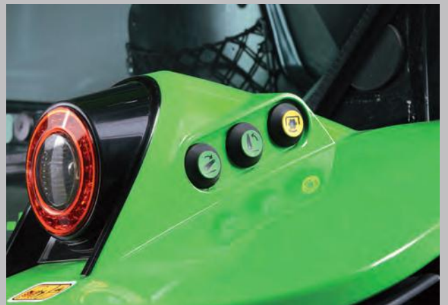
External PTO and rear lift controls for straightforward equipment mounting and external PTO operation.
