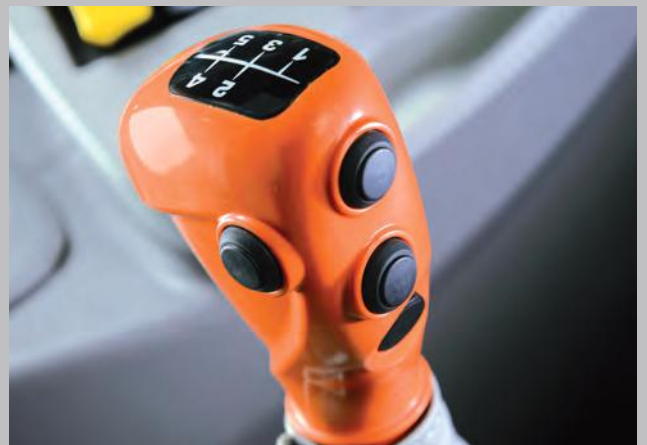
Bowden cables have made gear changing even more convenient at the push of a button.
