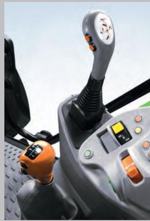
Front loader joystick with Powershift buttons. Stop&Go, SDD rapid steering system ...
