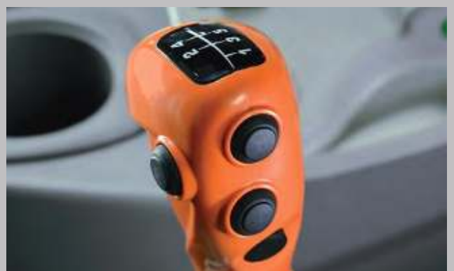
Comfort clutch and Powershift. Simply change gear at the push of a button without pressing the clutch pedal.
