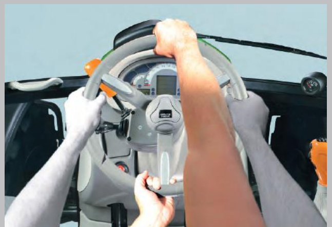
The SDD rapid steering system. Half the wheel rotation, double the steering power.
