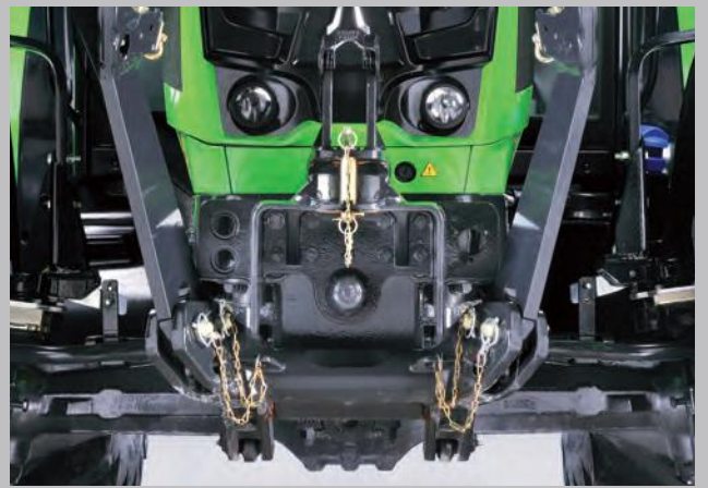
Front mounting points. Lifting capacity of 2,100 kg and 1000 PTO.
